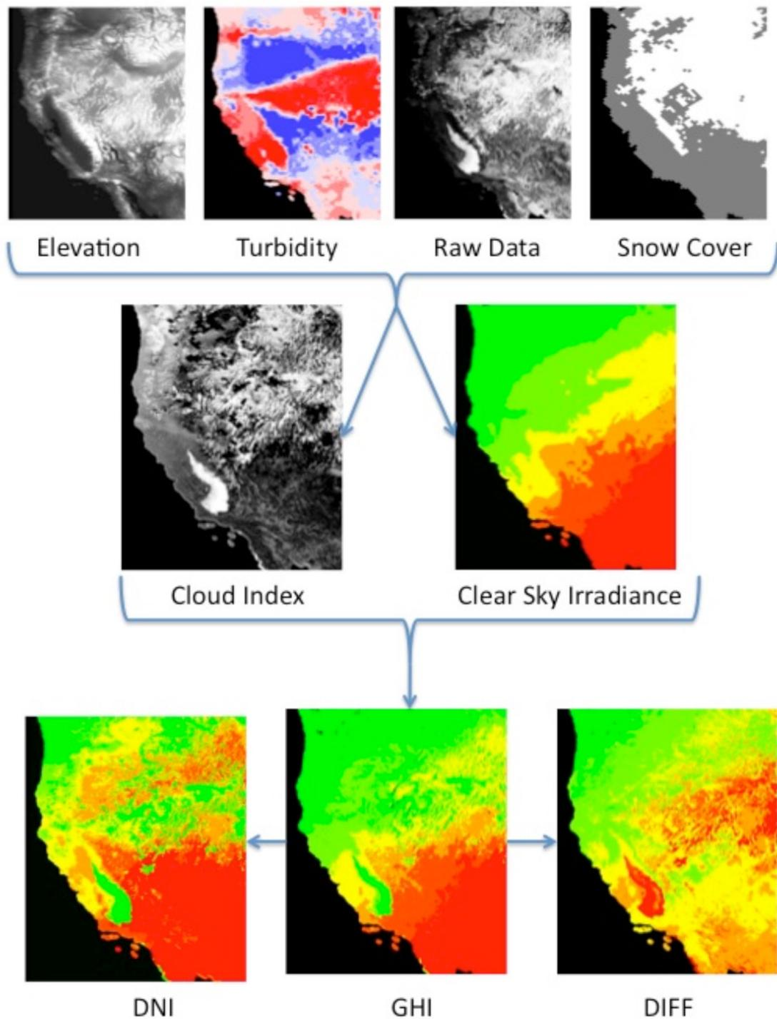
Figure 1. A flow chart showing 3TIER's method for calculating solar irradiance at the Earth's surface.
